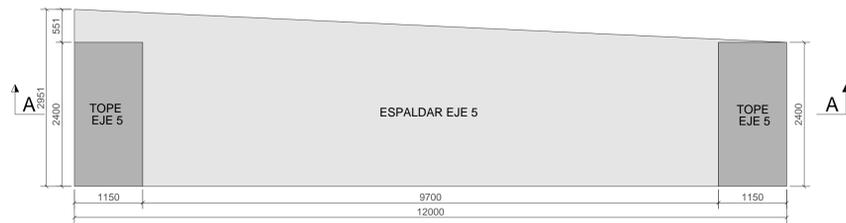
ALZADO - TOPE SISMICO Y ESPALDAR EJE 5
