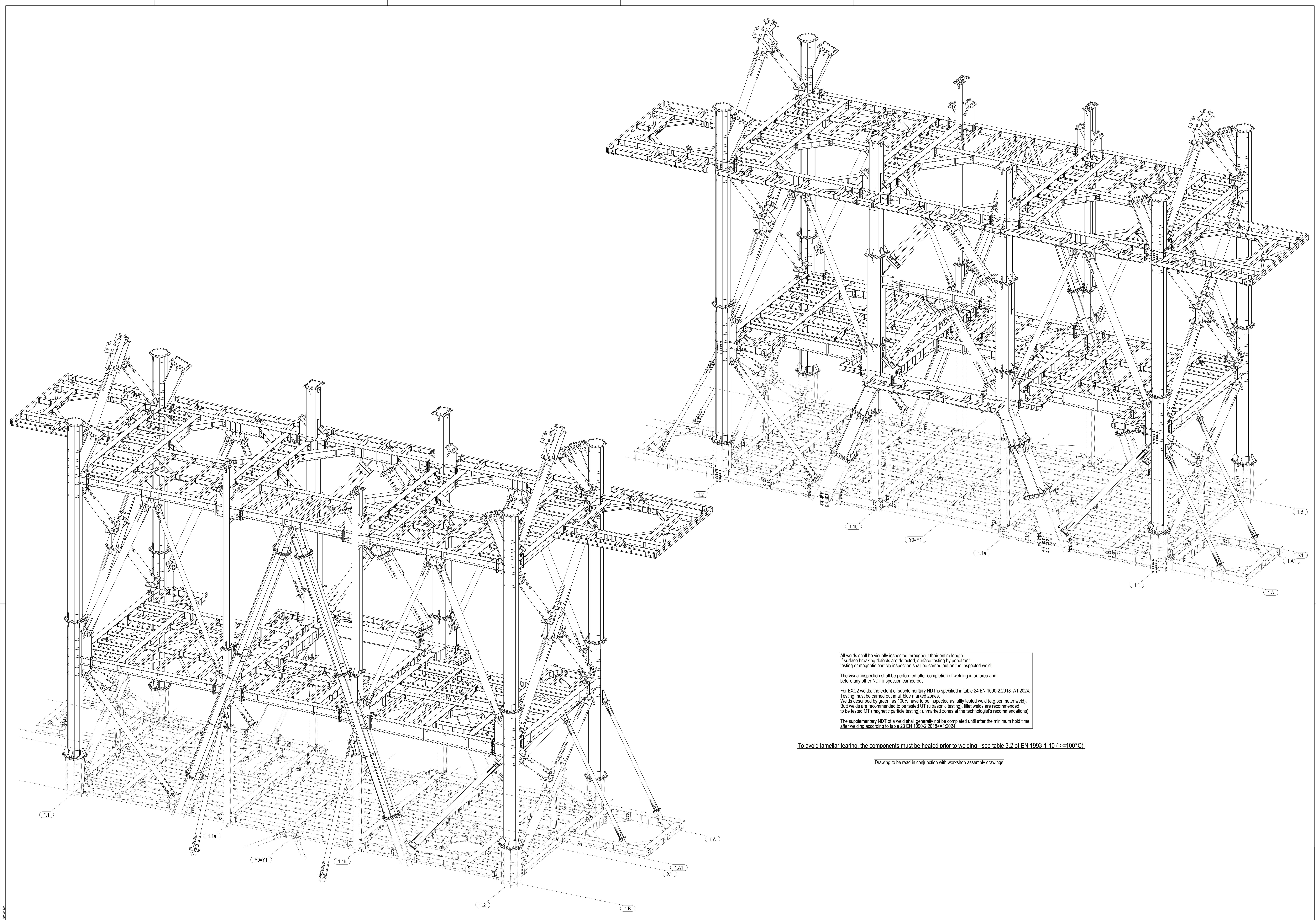
To avoid lamellar tearing, the components must be heated prior to welding - see table 3.2 of EN 1993-1-10 ( $\geq 100^\circ\text{C}$ )
